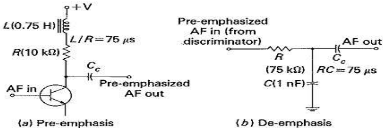
FIGURE 5-7 75-μs emphasis circuits.
